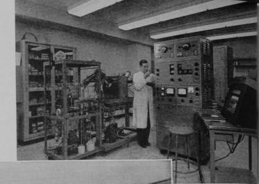
Mass spectrometer used in determining the absolute age of ancient rocks.
